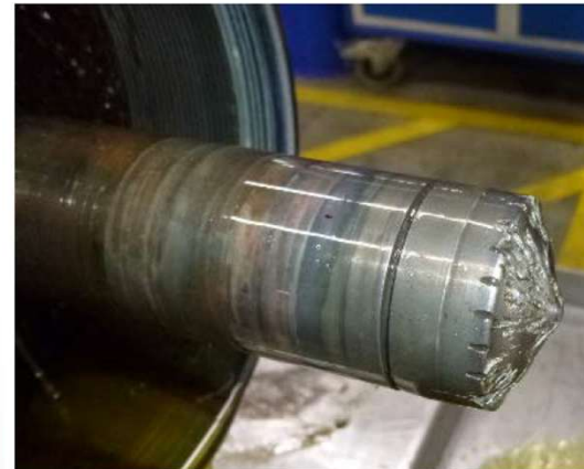
broken motor shaft (torsional oscillation in resonance with power supply)
