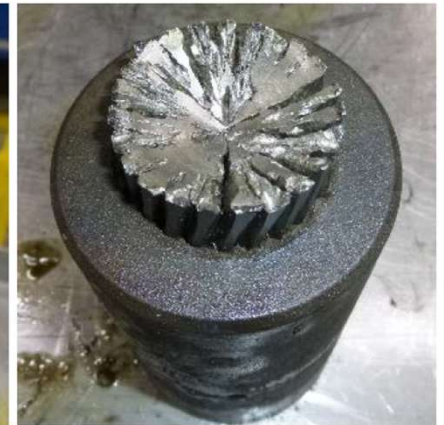
broken motor shaft (torsional oscillation in resonance with power supply)
