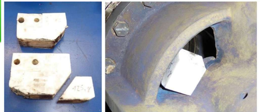
picture 30: reproduced Teflon piece fits through intake
