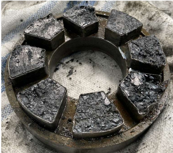
Shattered thrust bearing caused by pressure pulses
