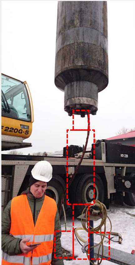
Broken ESP gauge (sensor)
