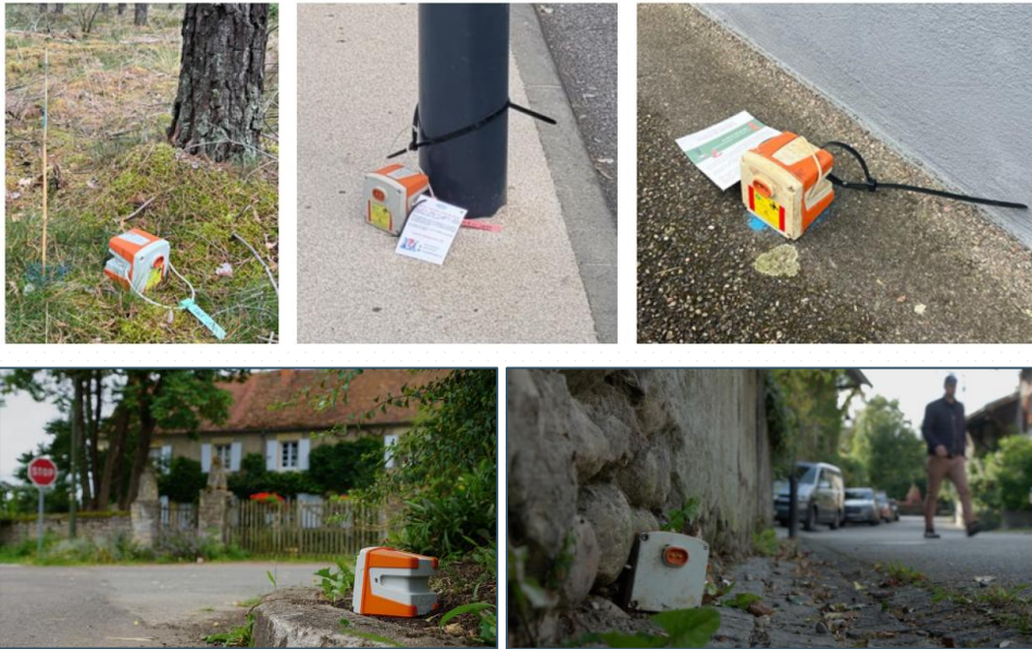
Examples of geophone placement
