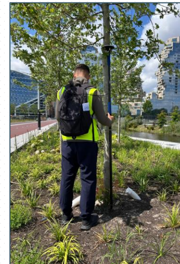
Shotpoint and receiver location surveying
