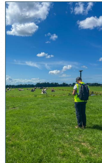
Shotpoint and receiver location surveying
