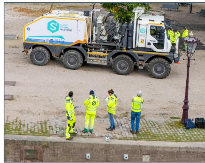
Vibroseis truck (large)
