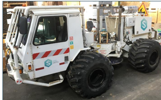
Vibroseis truck (small)
