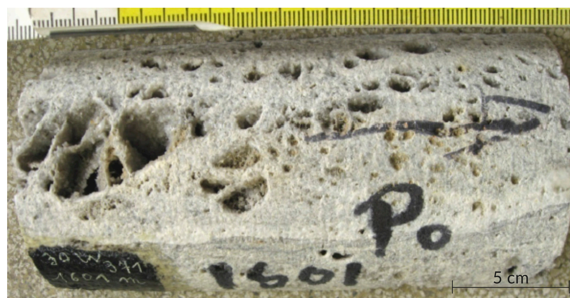
Figure 2. Core with karstified Dinantian carbonate rock from Belgian UGS well.
