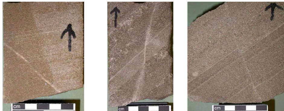
Figure 3-1 Examples of cataclastic faults in hand specimen. Fault displacements in the mm range are evident.
