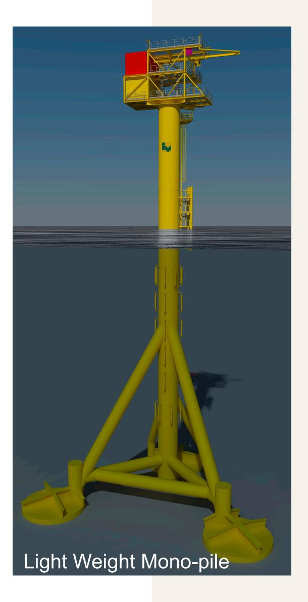
Simplified design stripped down to the bare bone suitable for shallow gas production
