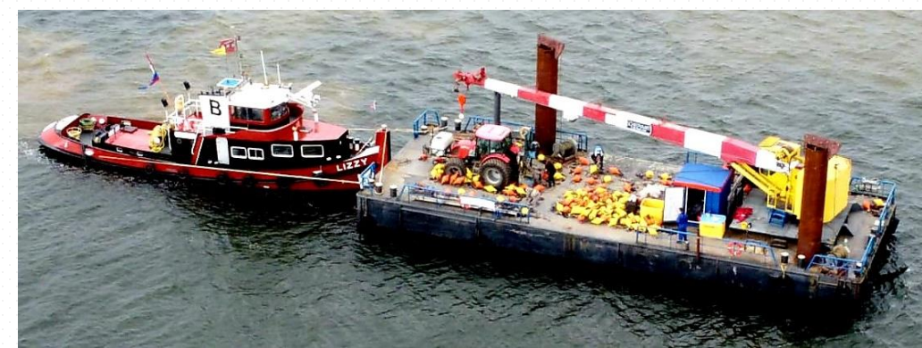
Barge/pontoon mounted drill tractor, usually 3 barges and 1 pontoon deployed, up to 58 shot points/day
