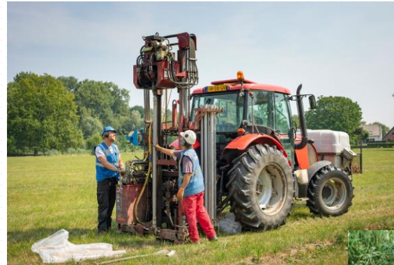
Land drill tractor, usually 5 tractors deployed, up to 100 shot points/day
