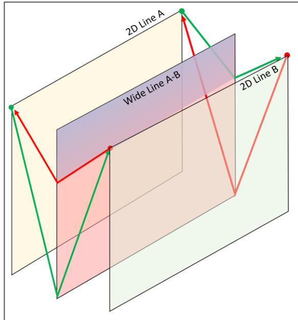
Figure 9 – Geometry of a wideline acquisition. Shots (green ray paths) of Line A are recorded on Line B and vice-versa (red ray paths), resulting is a new subsurface 2D line. Note there is no coverage of the shallowest part of the section due the too high angle of incidence.
