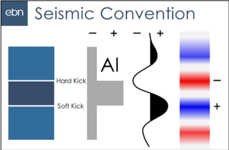
Figure 10 – Seismic convention used
