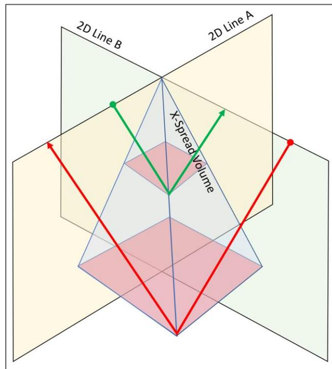
Figure 1 – Geometry of cross-spread acquisition for two perpendicular 2D lines. Shots (green ray paths) of Line A are recorded on Line B and vice-versa (red ray paths), resulting in a pyramidal shaped 3D volume (blue). The top of the pyramid is at the intersection of the two lines, the base of the pyramid is parallel to the 2D lines. Note that the shape of the 3D volume changes if more lines are included in the processing and/or if the lines do not intersect at a right angle.
