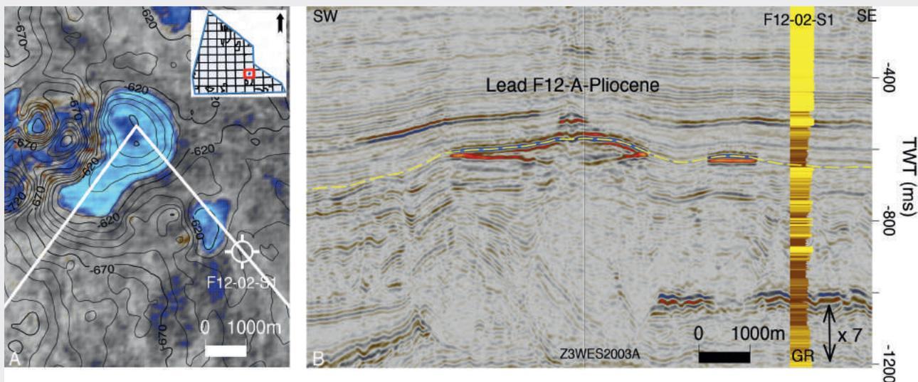
**Figure 11** A) Time map of the main reservoir of lead F12-A-Pliocene showing amplitudes. B) Seismic line through this four-way dip closure (location shown on Figure 11A). The top of the main reservoir is indicated by the yellow dotted line.
