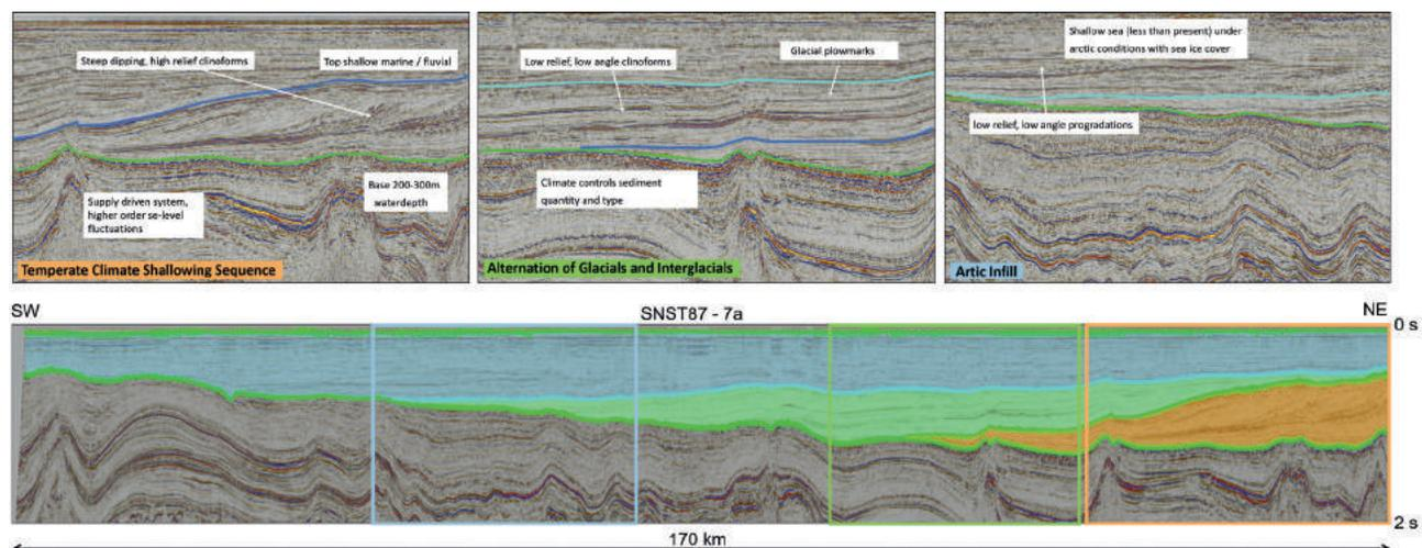
**Figure 6** Three depositional megasequences corresponding to specific paleoenvironmental conditions. Colours of the intervals correspond to those in Figure 4.
