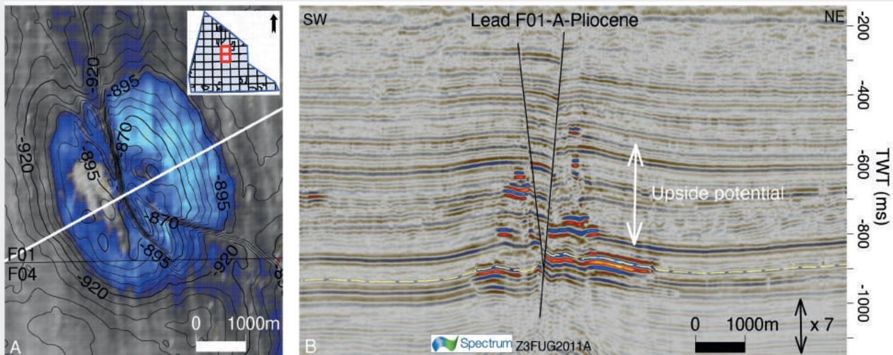
**Figure 10** Figure A) Time map of the main reservoir of lead F01-A-Pliocene showing amplitudes. B) Seismic line through this faulted dip closure (location shown on Figure 10A). The top of the main reservoir is indicated by the yellow dotted line.
