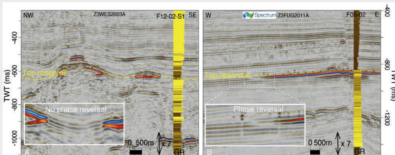
**Figure 5** A) Soft event (blue loop) at the top reservoir reflector (indicated by the yellow, dotted line) showing a strong decrease in acoustic impedance at the lead F12-A-Pliocene. B) The top reservoir reflector (indicated by the yellow, dotted line) showing a strong decrease in acoustic impedance resulting in a phase reversal at the gas lead in quadrants F04-F05.
