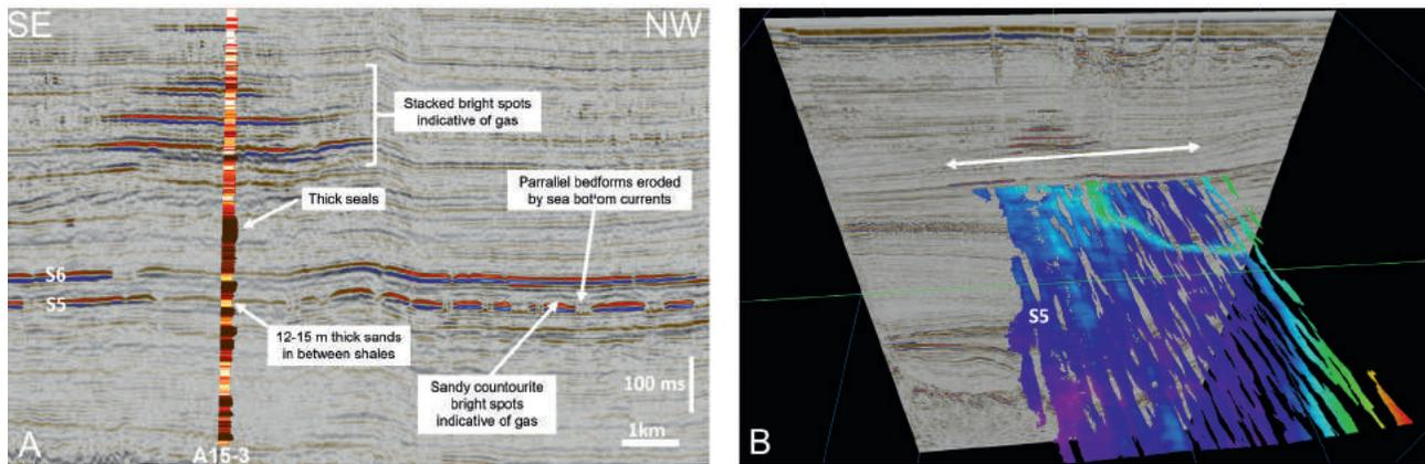
**Figure 7** A) Sandy contourite type bright spots in S5 and S6. B) Auto-tracked high amplitude reflections associated with sandy contourites of S5.
