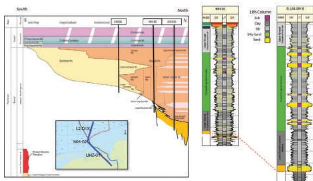
**Figure 5** Upper Rotliegend stratigraphy architecture adapted to reflect the new geological model (after Van Adrichem Boogaert, and Kouwe, 1993-1997 and Schröder et al., 1995).
