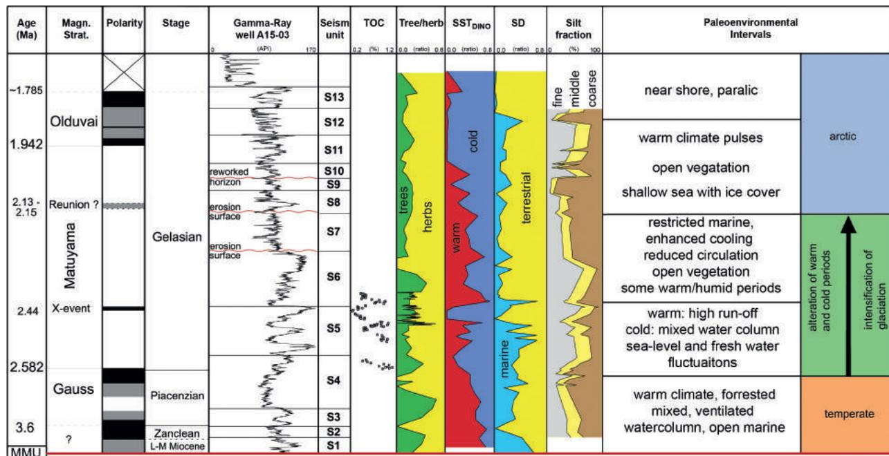
Figure 4 Correlation and interpretation of chronostratigraphy, Gamma-Ray log, seismic units, geochemical and palynological proxies, grain size. Data from Kuhlmann et al. (2006), Kuhlmann and Wong (2008), Donders et al. (2018) and Ten Veen et al. (2013).
