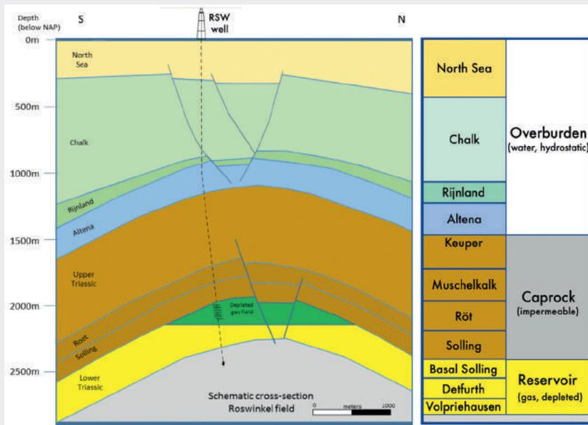
**Figure 2** Schematic cross-section of the Roswinkel field, incl. overburden. The stratigraphic chart defines further which formations can be generally grouped into reservoir, caprock and overburden with associated fluid fill and evaluated pressure regime, respectively.
