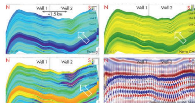
**Figure 3** Cross-section from the static reservoir model from well 1 to well 2 displaying porosity (top left) and net to gross ratio (top right). The predicted acoustic impedance from the reservoir model (bottom left) and synthetic seismic data (bottom right) show the strong lateral changes porosity and NiG ratio, which are inconsistent with the actual seismic data (backdrop).
