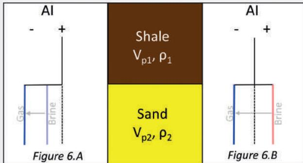
**Figure 6** Schematic explanation of Figure 5A and B showing a case in which substituting brine with gas in the reservoir sand results in an amplitude decrease only (left) and a case in which this results in a phase reversal (right).
