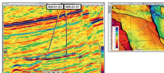
**Figure 6** Line through N05-01-S1 and S3 on the coloured inversion volume. Both wells display gamma ray curves. Inset map is top reservoir depth surface.
