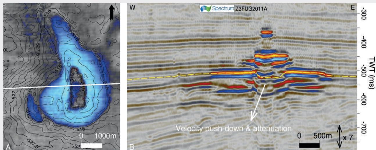
**Figure 9** The combination of velocity push-down and attenuation gives rise to the doughnut effect: an artefact that is fairly typical for stacked shallow gas occurrences in the Netherlands.
