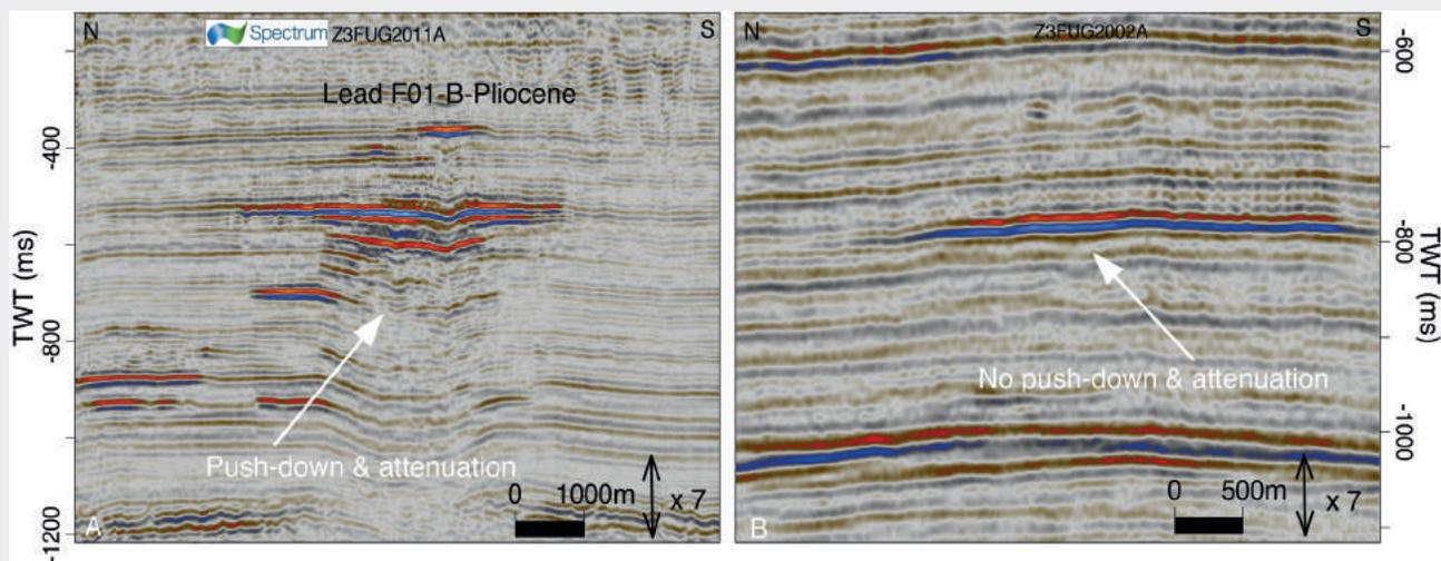
**Figure 8** A) Amplitude anomaly in quadrant F01 with a push-down effect, increasing with depth. Also attenuation of the seismic signal is observed. B) Amplitude anomaly in quadrant B14 that does not show a push-down effect nor attenuation.
