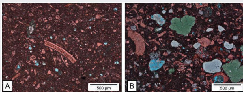
**Figure 3** Well F17-11: Thin sections of Upper Maastrichtian clean chalk (A, MD depth xx42.6 m), Lower Maastrichtian sandy chalk (B, MD depth xx77.6 m). Depths are deliberately masked for confidentiality purposes, but compare to Figure 2. Note that the chalk mud matrix is dark in these thin sections; the around 45% microporosity in the chalk mud is not resolved in the thin section.
