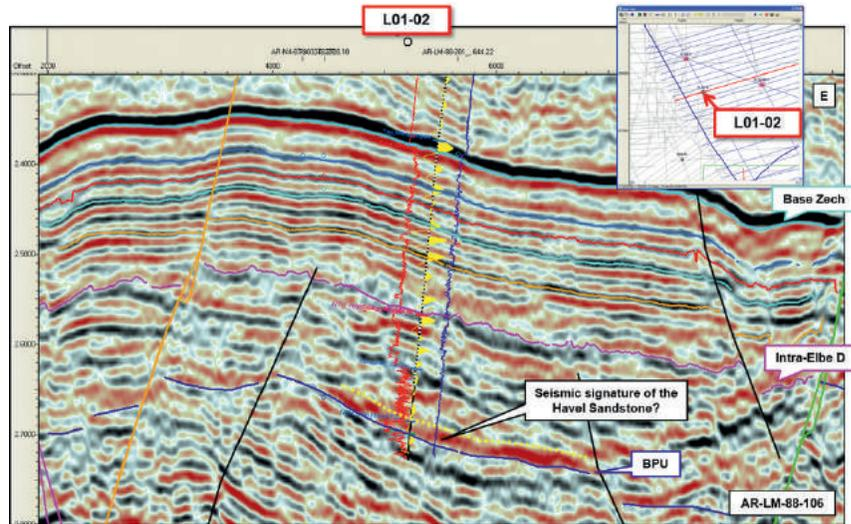
**Figure 3** L1-2 well drilled in Germany shows the sands corresponding to a low acoustic impedance unit, the mapped negative (red) interval on the coloured inversion (after Corcoran and Lunn, 2014).
