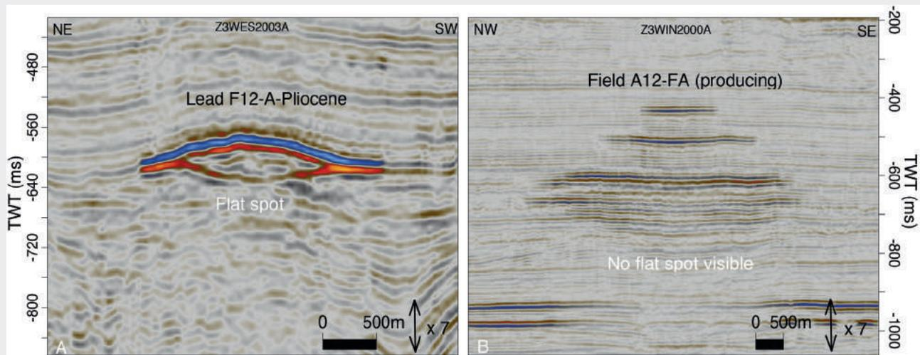
**Figure 7** A) Amplitude anomaly F12-A-Pliocene with a clear flat spot, indicative of a GWC. B) No flat spots are visible in producing field A12-FA.
