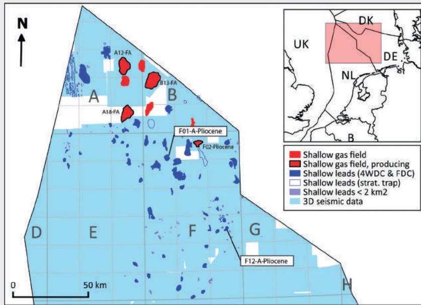
**Figure 1** Study area showing the eight shallow fields (red), of which four are currently producing (black outline), and the identified shallow leads. Case study 1 (F01-A-Pliocene) and case study 2 (F12-A-Pliocene) are also indicated. The 3D seismic data coverage in the area is shown in blue.
