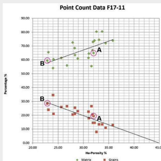
**Figure 4** Point Count Results of F17-11 thin sections. Chalk porosity increases with increasing amount of matrix (Note: the mud matrix also contains the microporosity) and decreasing amount of grains (skeletal and siliciclastic grains). Samples Figure 3 marked by circles A and B.
