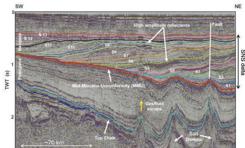
**Figure 2** W-NE seismic cross-section (see Figure 1 for locality) showing the westward prograding Southern North Sea delta of Plio-Pleistocene age. Seismostratigraphic units according to Kuhlmann et al. (2006).
