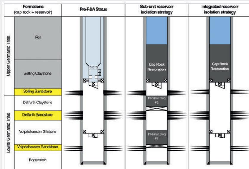
**Figure 3** Schematic well status diagram with respect to reservoir units and stepwise improvement of zonal isolation at Roswinkel.
