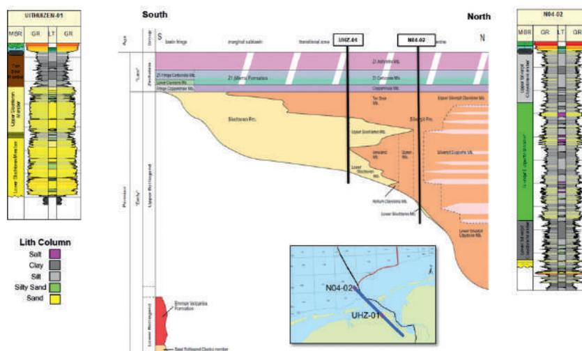
**Figure 2** Upper Rotliegend stratigraphy architecture. The previously published stratigraphic model indicates that Hansa's acreage (now ONE's) in the Dutch sector is shale prone (after Van Adrichem Boogaert and Kouwe, 1993-1997).
