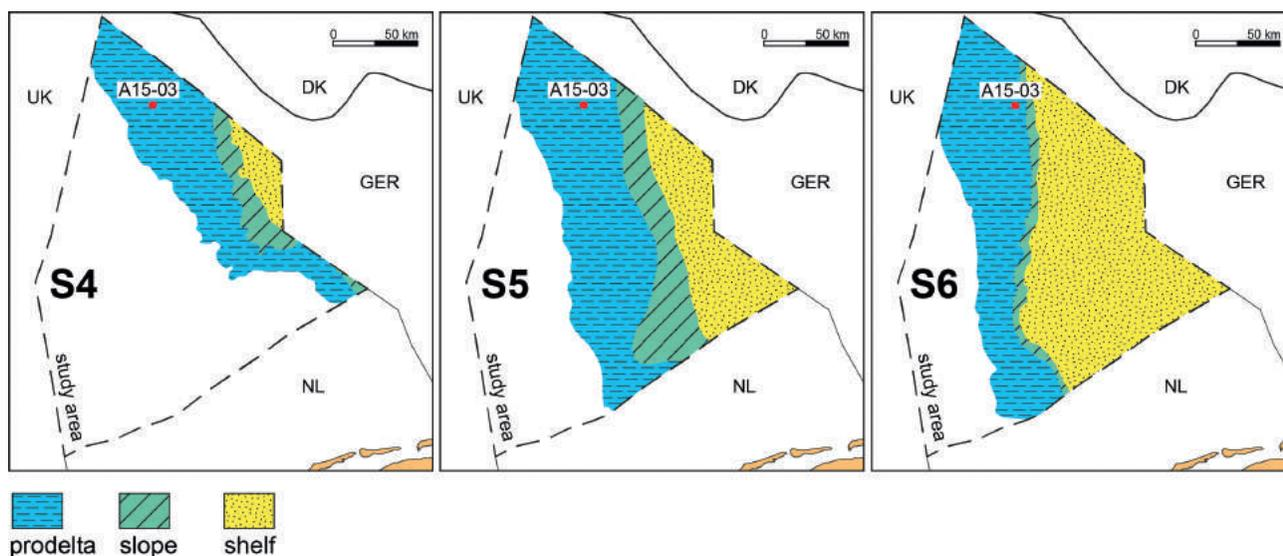
**Figure 3** Regional distribution of shelf-prism clinoform elements through time, with shelf (yellow), slope (green) and basin floor (blue) for units S4-S6 showing the regional distribution of delta elements (delta evolution) through time.
