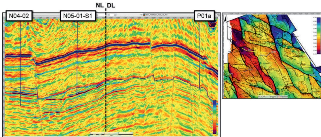
**Figure 4** The basal Rotliegend sand can be mapped from Germany into the Netherlands where the reservoir is proven. No low acoustic impedance body is mapped at N04-02 where only thin basal Rotliegend Sandstones were encountered. Inset map is top reservoir depth.
