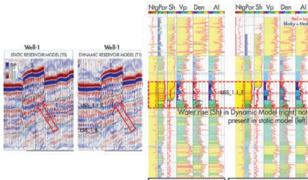
**Figure 4** Subtle differences in synthetic seismic data based on initial (T0, left-hand seismic section) and on depleted reservoir conditions (T1) (right-hand section) reveal a rising contact owing to production of hydrocarbons. The same effect is shown in the log panels to the right.
