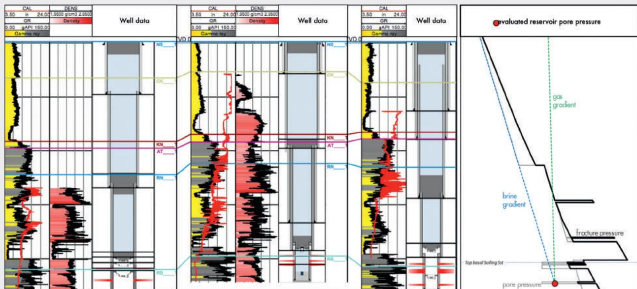
**Figure 4** Integrated data visualization on geological, petrophysical, well engineering and geomechanical data. Only three wells are shown as examples. During the Isolation strategy session all wells are plotted and discussed. Note that the mechanical well data is reflecting the final isolation status, including cement plugs across the full wellbore diameter. The focus of this article is on the reservoir isolation.
