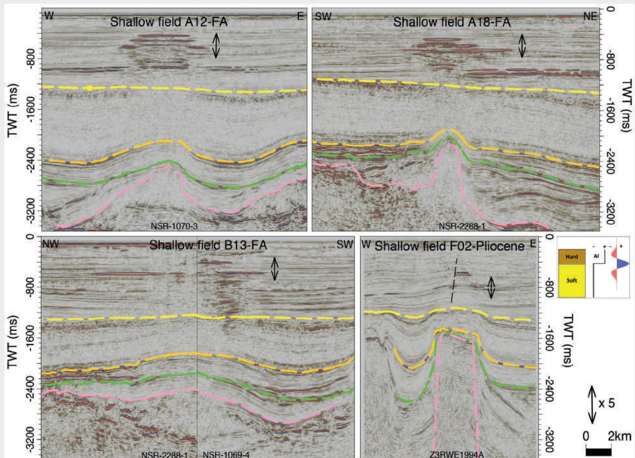
**Figure 3** Seismic lines through four producing shallow gas fields in the Netherlands (location indicated on Figure 1). The arrows indicate the producing reservoirs. The Base Upper North Sea Group (yellow), Base North Sea Group (orange), Base Chalk (green) and Top Zechstein (pink) are indicated.
