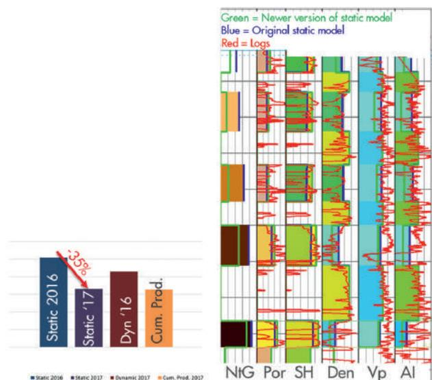
**Figure 2** Left: GIIIP estimates derived from static models in 2016 and 2017, and a dynamic model from 2017, compared to cumulative production at the end of 2017. Right: Well panel with logs in red indicating net-to-gross (NiG), porosity (Por), hydrocarbon saturation (SH), density (Den), velocity from sonic (Vp), and acoustic impedance (Ai). Original 2016 model results in blue and updated 2017 model in green.
