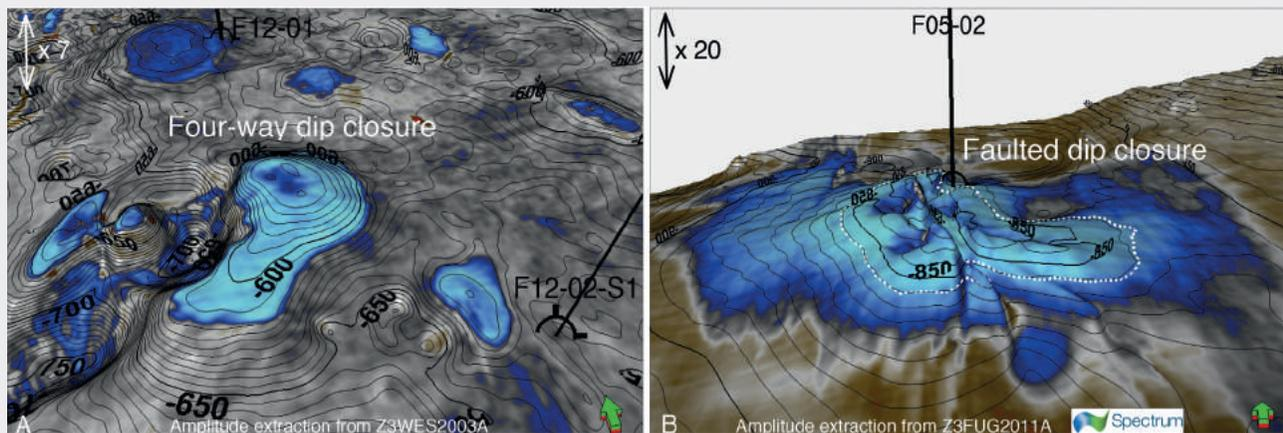
**Figure 4** A) Amplitude extraction plotted on the top reservoir map (TWT) of a four-way dip closure bright spot (area 5 km<sup>2</sup>). B) Amplitude extraction plotted on the top reservoir map (TWT) of a faulted dip closure bright spot (area 40 km<sup>2</sup>). The white stippled line indicates the brightest part of the anomaly that is conforming to structure.
