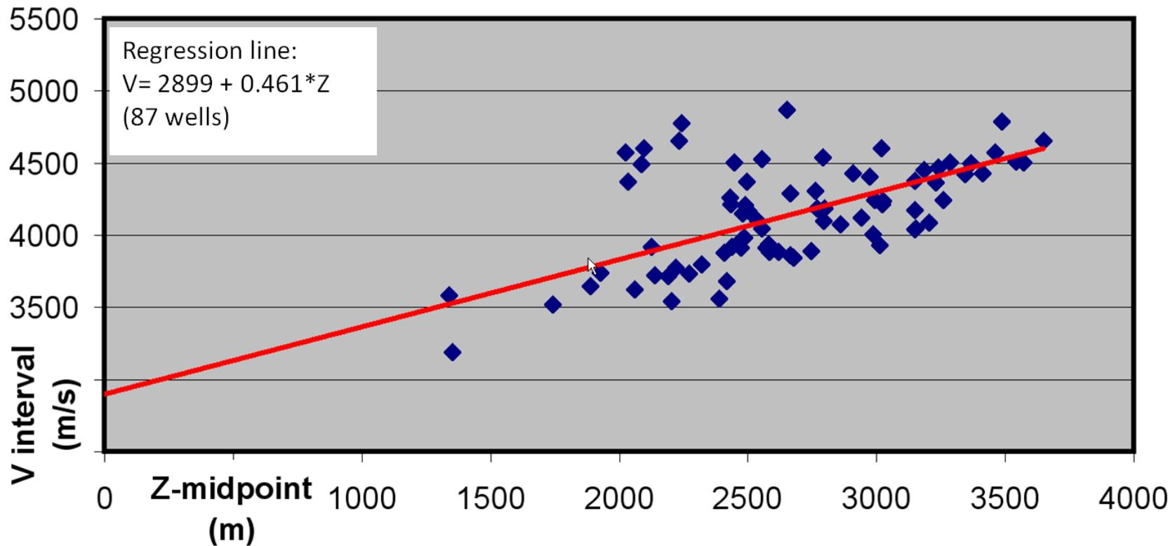
Interval velocity vs midpoint depth plot (Lower Bunter)
