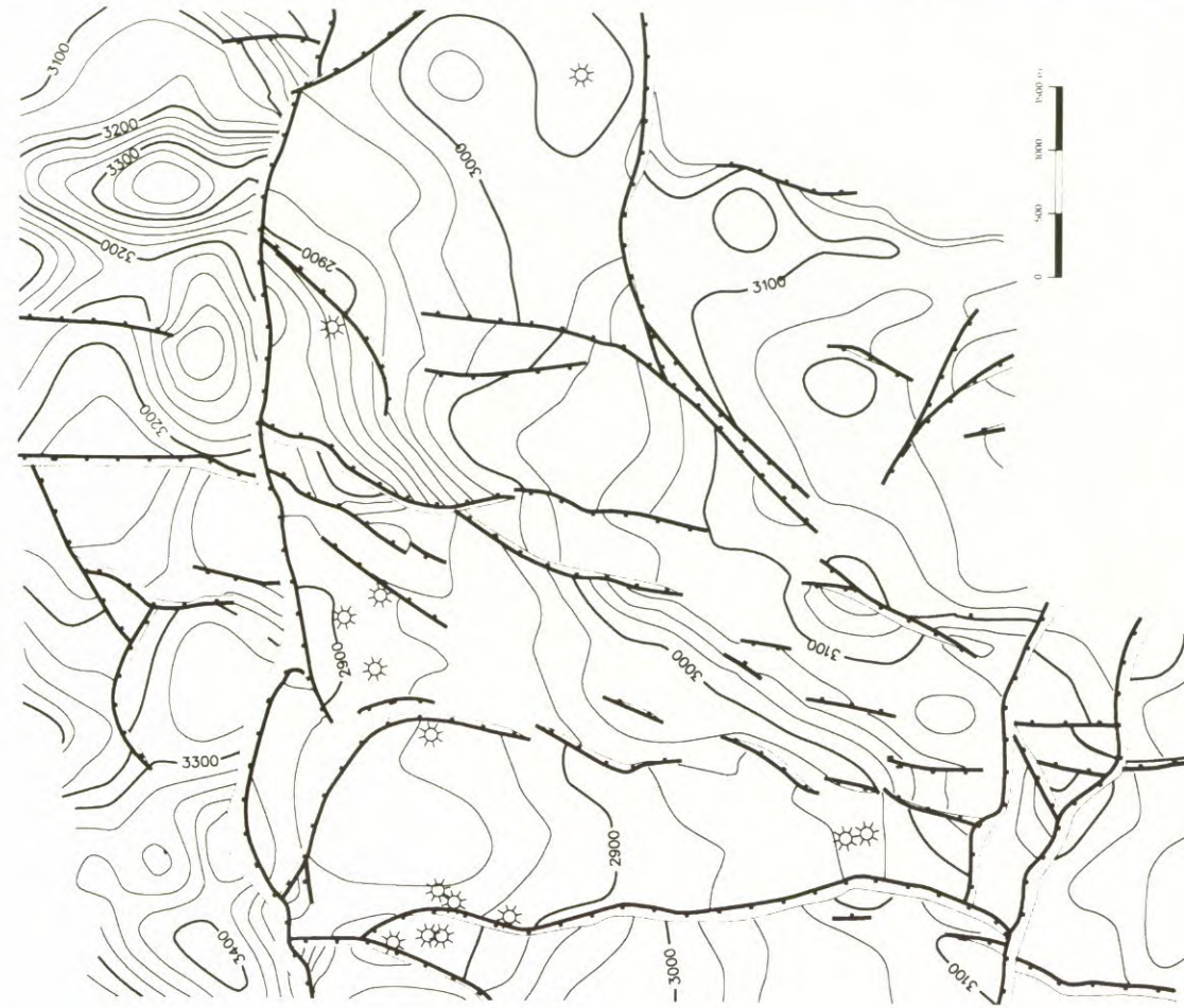
Fig. 10. Depth structure map over the centre of the Annerveen Field for the top Rotliegend reservoir horizon: 1989 interpretation.
