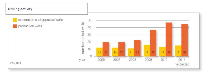
A total of 13 exploration and appraisal wells were drilled in 2010. Consisting of nine exploration wells, of which two were onshore. The total new volumes discovered by both exploration and appraisal wells amounted to 7 BCM. Excluding appraisal wells, the success ratio of exploration drilling was 67%, which is exactly the same as in 2009.
