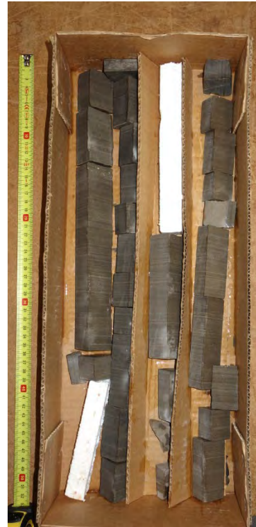
Laminated/varved nature of the Hauptdolomit at the top of the core. 2188m (top left) – 2190m (bottom right)
