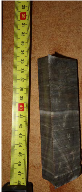
Interval with laminated anhydrites/ dolomitic limestones. 2190.35m
