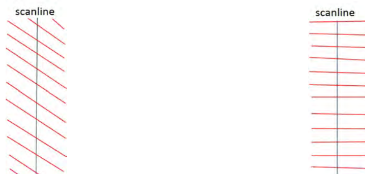
Figure 5.5: Effect of scanline orientation with respect to fracture set. Scanline perpendicular to fracture set; # fractures = 12, scanline 45° to fracture set; # fractures = 10.
