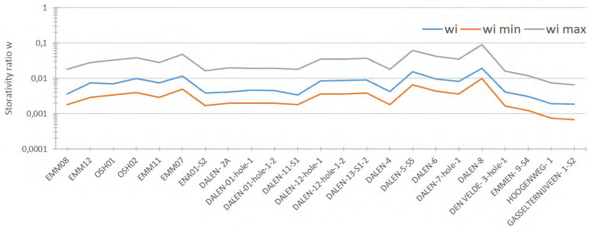
Figure 5.3: Storativity ratio \omega boundaries ( w_{i\ min} and w_{i\ max} ) and the storativity ratio w_i calculated using the Warren & Root model.
