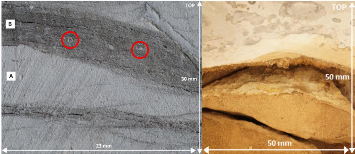
Figure 4.3 – **Left:** Homogeneous chalk (A) with a dark contrast clay wavy layer (B) in between from HRL-02 core, top depth 1078.6 meter. Red circles indicate macro fossil debris in the dark contrast layers. **Right:** Oil up to contact in the F06-02 well, where the lower part of the image is oil stained homogeneous chalk and the top part is a flint nodule/layer.
