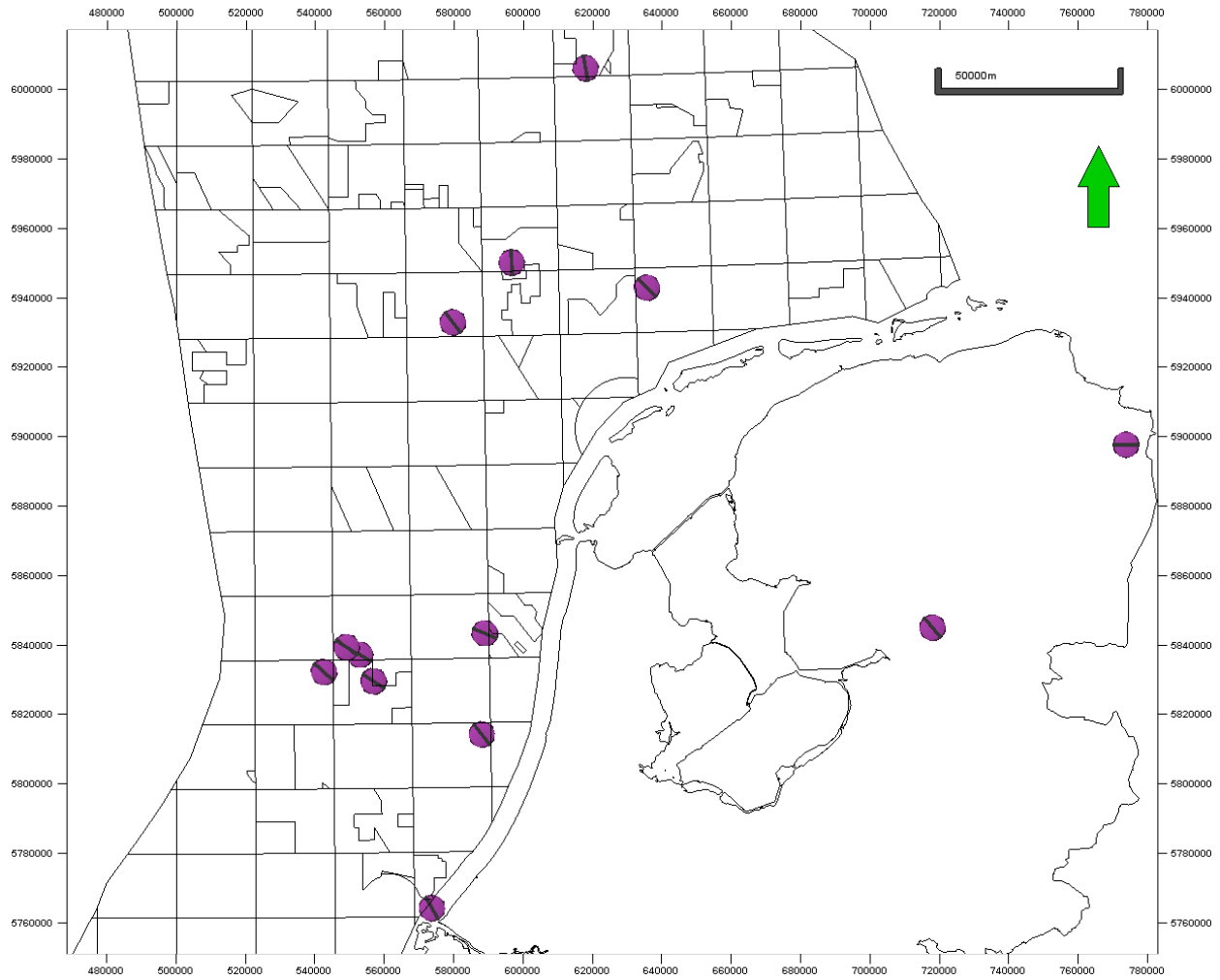
Figure 55: Dutch Stress Map indicating for each well the average S_H direction in the Lower Germanic Trias Group.
