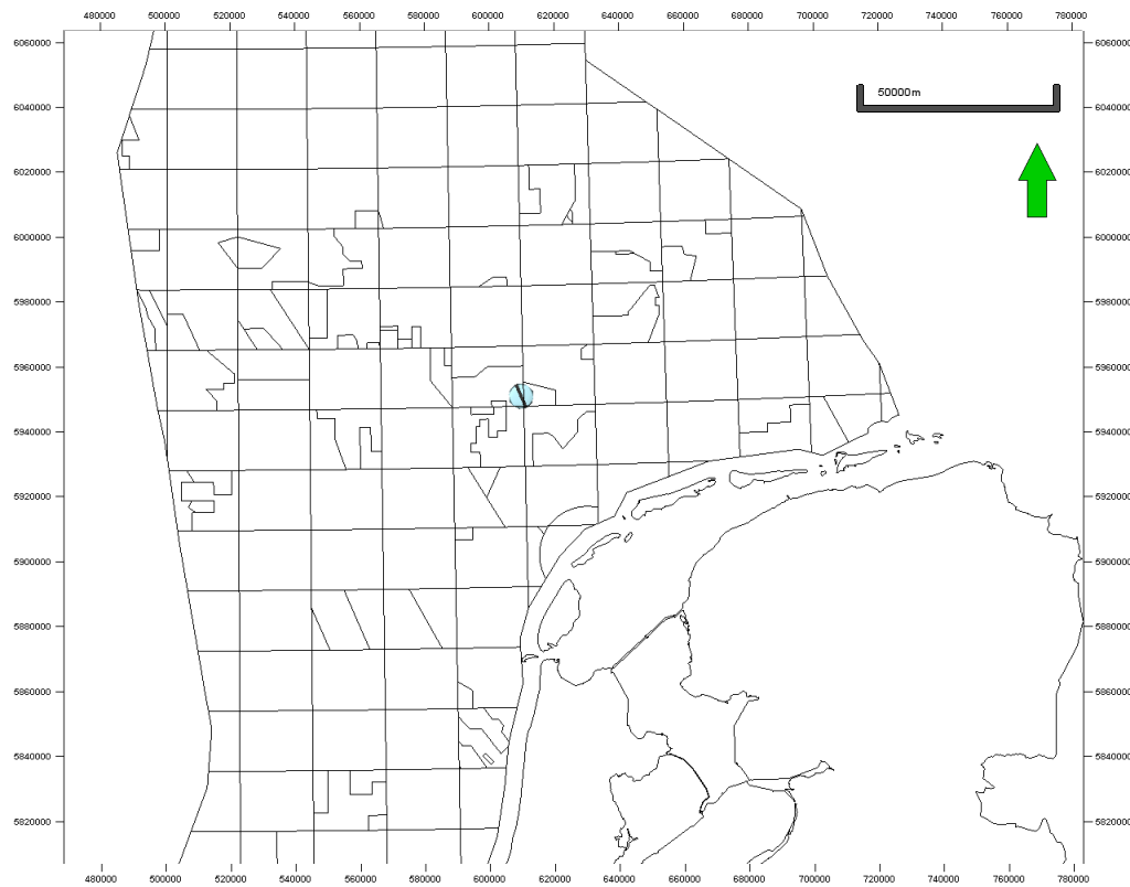
Figure 53: Dutch Stress Map indicating for one well the average S_H direction in the Schieland Group.
