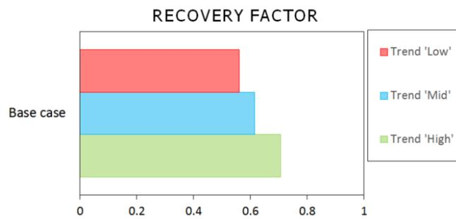
Figure 4.10: Recovery factor resulting from the reservoir simulations with the defined rock compaction trends.
