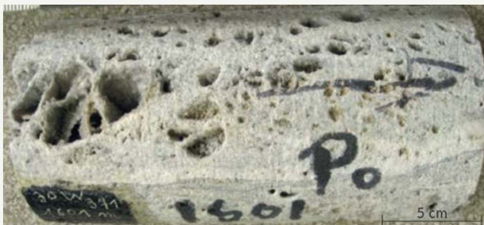
Core with karstified Dinantian carbonate rock from Belgian underground gas storage well
